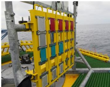
**Advanced floating platform for the evaluation of standardized probes and components in real offshore environment**
