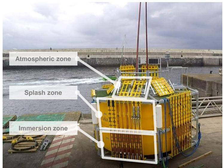
HarshLab1.0 is suitable to test new materials and solutions against corrosion, ageing and fouling in real and monitored offshore conditions
