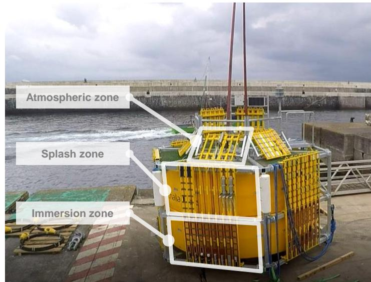
**HarshLab1.0 is suitable to test new materials and solutions against corrosion, ageing and fouling in real and monitored offshore conditions**
